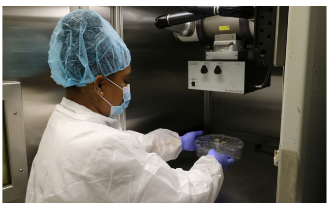
(left) The XRad320 X-ray irradiator delivers precise dose to specimens and allows for quick changes between total body radiation and focal radiation treatment. (right) Additionally, cesium-137 is available for low-dose application for cell imaging.
